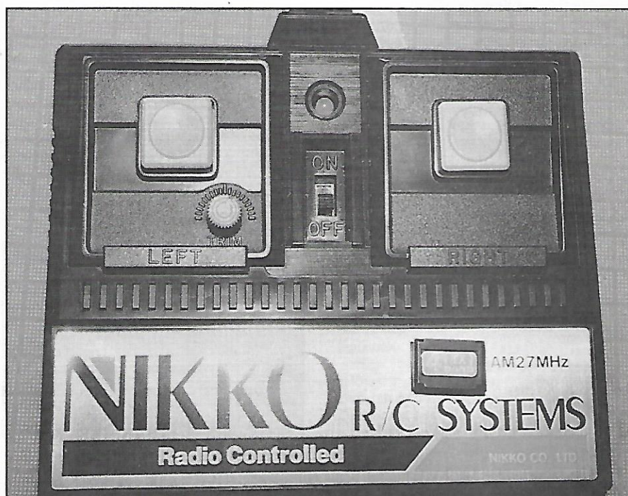
Nikko transmitter is as simple as you could wish for. Knob adjacent to 'left' button is for rudder trim.
