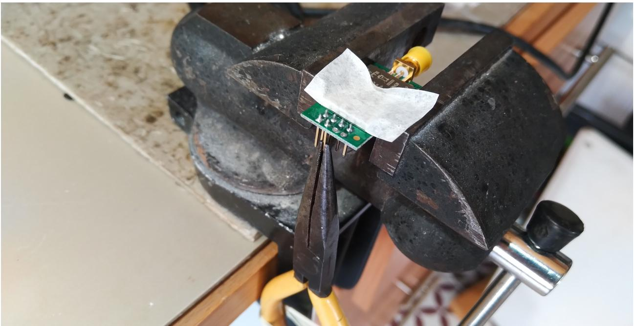
The 'de-pinned' NRF should look like this with nice clean holes. If not, you might struggle to get the connection wires through:
