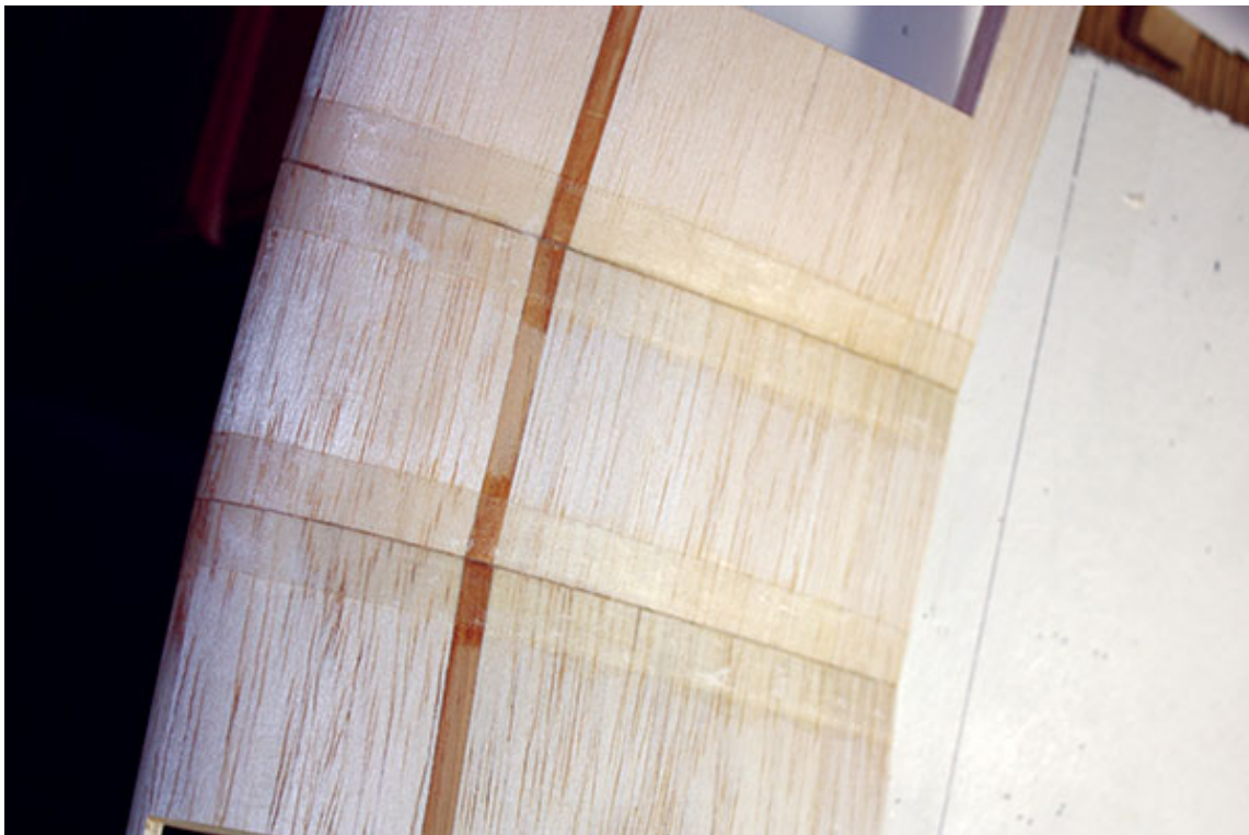
05. The Fidget's outer wing panels are buttglued to the center panel. The joints are wrapped with 1-inch fiberglass tape applied with CA glue.
