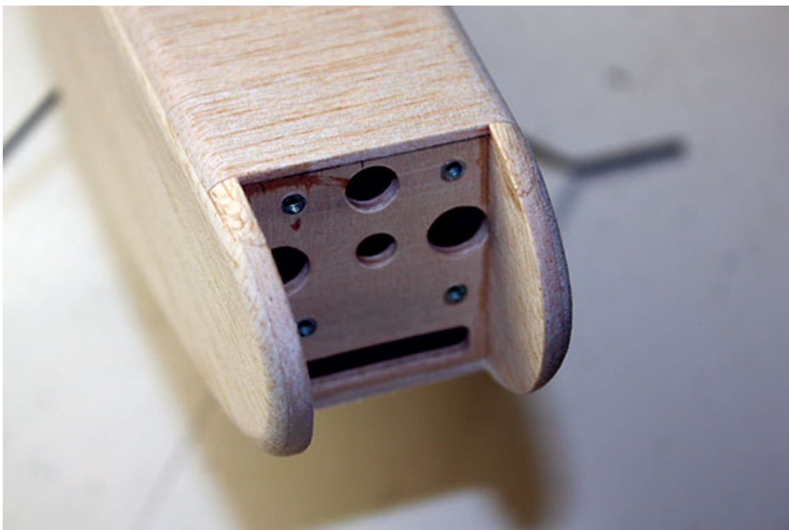
07. The firewall has 4-40 blind nuts and air-cooling holes. Also shown are the 1/8-inch balsa fuselage nose doublers and upper scrap-balsa fill-ins.
