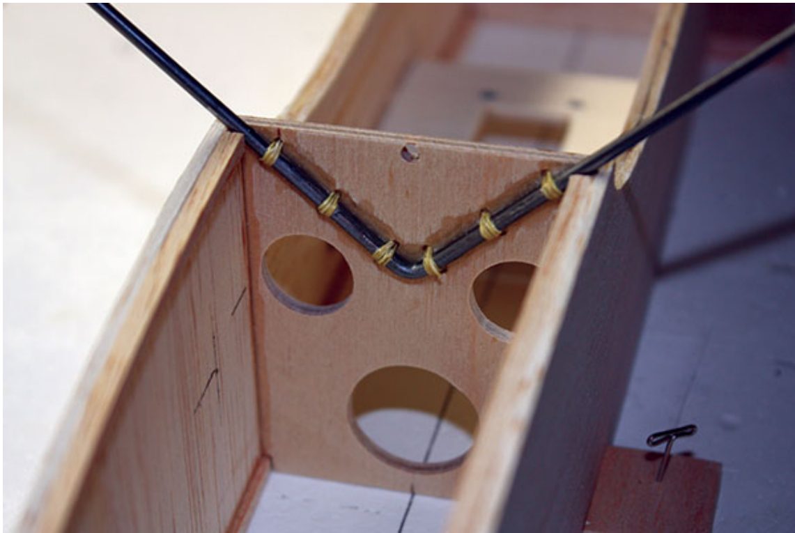
01. The 3/32-inch diameter music wire landing gear is attached to former F2 with Kevlar fishing line and CA glue. Note the hole for the wing dowel and air-cooling holes.
