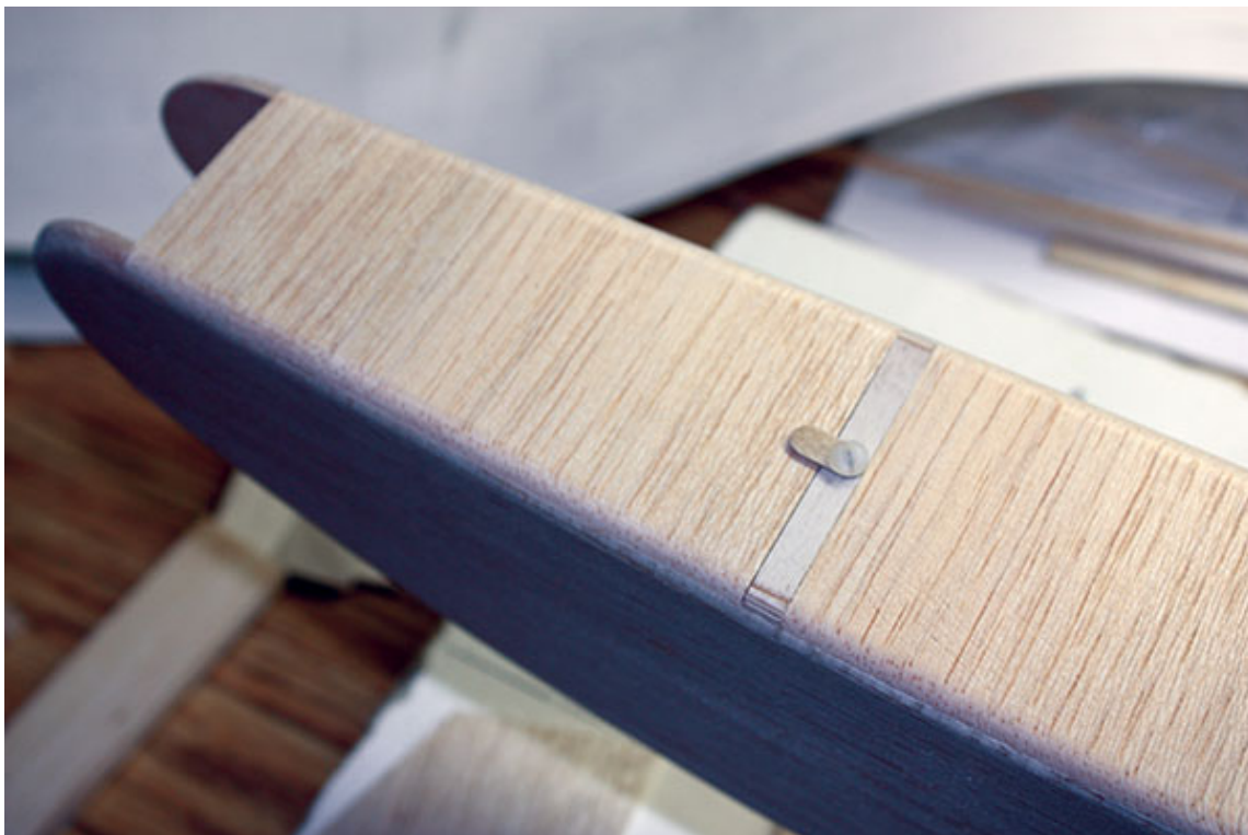
06. The hatch lock is made from 1/32-inch plywood and attached with a 4-40 nylon screw to adjust friction.
