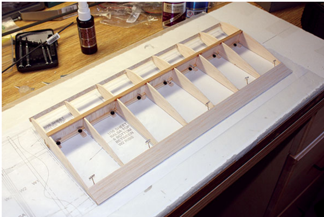
04. The right wing panel is nearly complete. The 1/16-inch balsa sheeting still needs to be added to the inboard rib bay at the left end of the wing panel.
