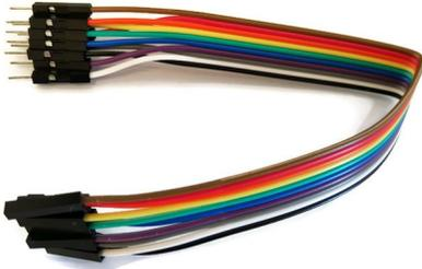
If you're going to use the programming lead repeatedly, you can glue the connectors together at each end to form plugs and sockets suitable for connection to the gyro and your USBasp. Use a tiny amount of superglue, and be careful not to accidentally permanently glue the leads into your USBasp socket!
